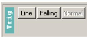
Setting the trigger source (CH1 – CH2 – Line) and mode (Rising–Falling and Normal - Single) is possible on the "Trig" panel. Selecting CH1 or CH2 makes the trigger sensitive for that channel. If the source is set to "Line", the signal processing takes place without triggering. The "Falling" and "Rising" options make the trigger sensitive to the edge selected. In Single mode must be set timeout for single triggering.
